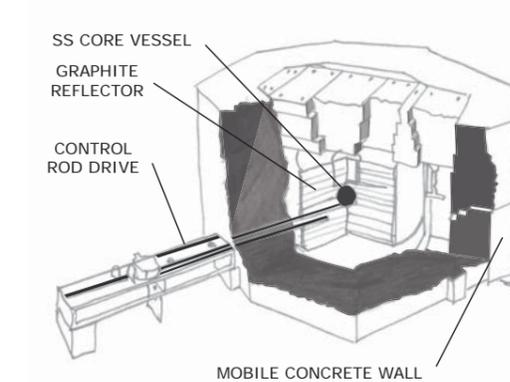
**The DR1 reactor at what is now called Risø National Laboratory, Technical University of Denmark – DTU.** It was commissioned in 1957, taken out of service in 2001 and decommissioned by Danish Decommissioning in 2004-05. The reactor was a thermal homogeneous reactor with an output of 2 kW. The fuel was 19,9 % enriched uranium in the form of uranyl sulfate dissolved in light water. The core comprised a spherical vessel having a diameter of 0.32 m.
