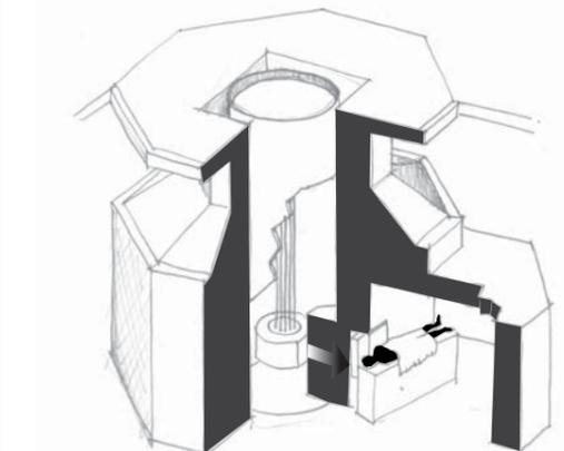
**The TRIGA research reactor at VTT in Finland** has been in operation since 1962. The uranium fuel is enriched to 20 % and it is moderated by light water. The power output is 0,25 MW. The present operation is mainly for Boron Neutron Capture Therapy.
