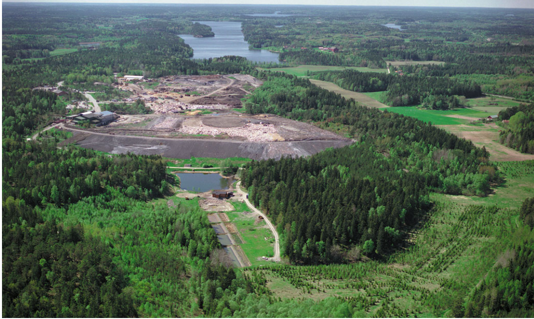
Figure 1. Aerial photo of the Tveta Landfill Site with slope to be covered, leachate pond, purification plant and wetlands. In the foreground the forest for the irrigation system
