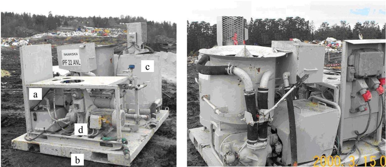
Figure 2. Equipment for the injection tests: pumping platform with a 150 litres mixing tank (a), high pressure jet mill (b), equalization tank (c) and piston pump (d).
