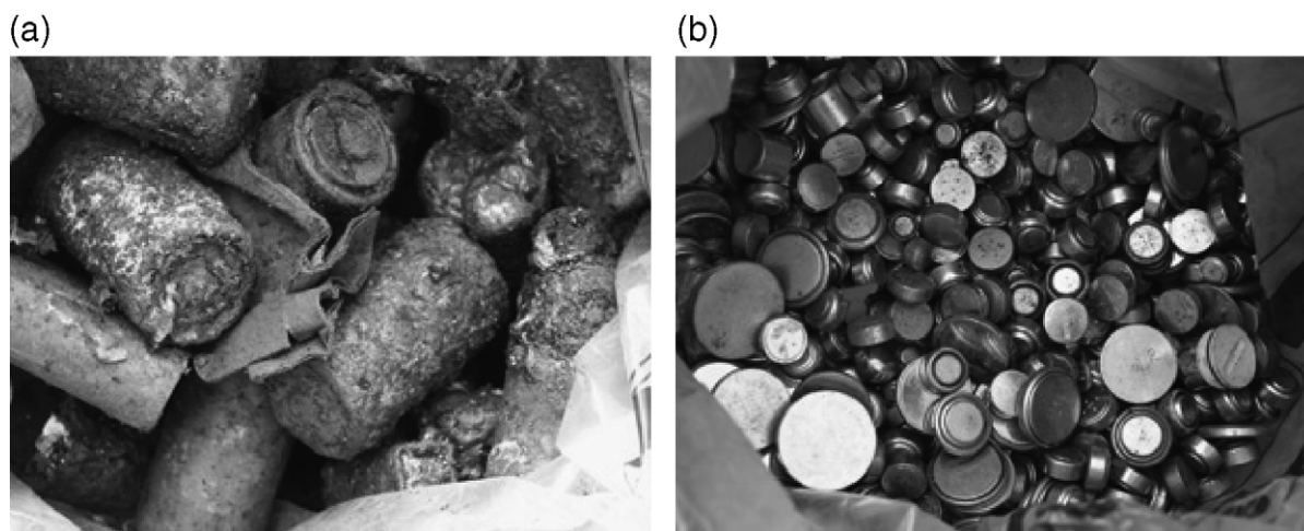
Fig. 3. Sample material for the present project. (a) Unsorted batteries. (b) Zinc-mercury oxide batteries.
